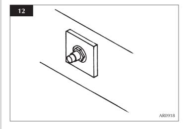
8.4 Holding the injector with a spanner, undo the feed pipe. **NOTE: THE ORIENTATION OF THE INJECTOR.**
